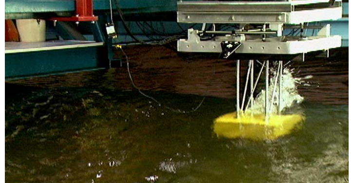
Figure 1: Captive setup for force measurement on block (left) and the situation in the basin (right).
